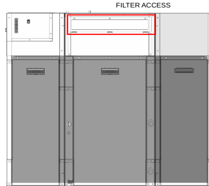
Figure 5 – Air filter location
